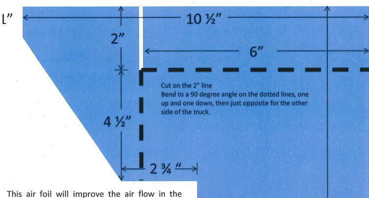
This air foil will improve the air flow in the back of the truck, preventing the buildup of snow and dust. It will also improve the visibility for the motoring public when approaching snow plows from behind by keeping the strobe lights, turn signals and reflective material more visible.
