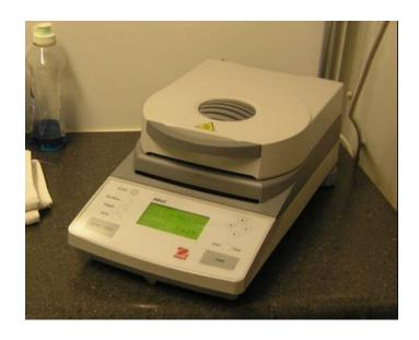
The moisture balance used should have a capacity of 35g and a minimum readability of 0.005g. Set up the moisture balance according to the manufacturer's recommendations. Operate instrument in an automatic mode for the stop point and at 160 C drying temperature. Place approximately 25 g on the sample pan and press start. Record the % moisture at completion of the test.
