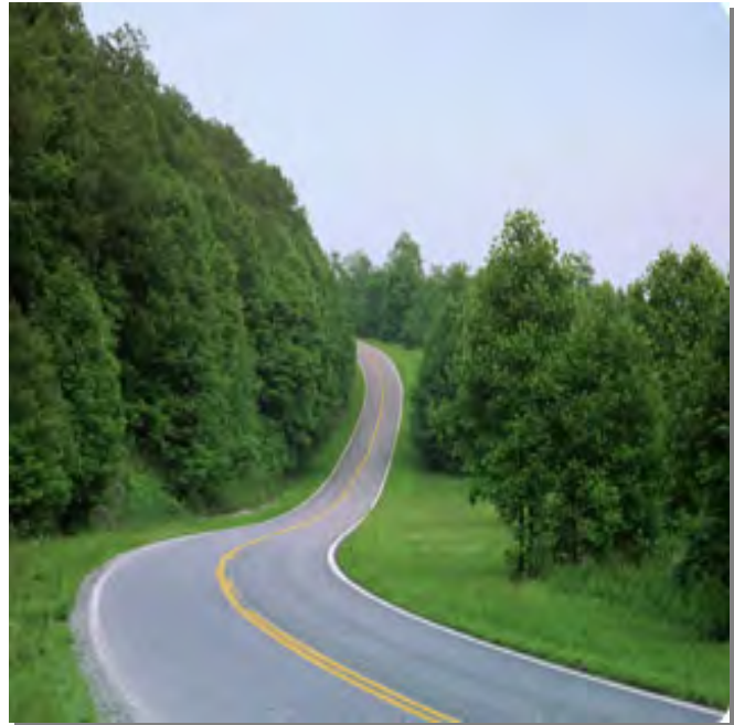
Figure 8-4. Woody Vegetation in Roadsides - provides cover for deer and increases the risk of deer-vehicle collisions (Photograph: BASF Professional Vegetation Management.)
